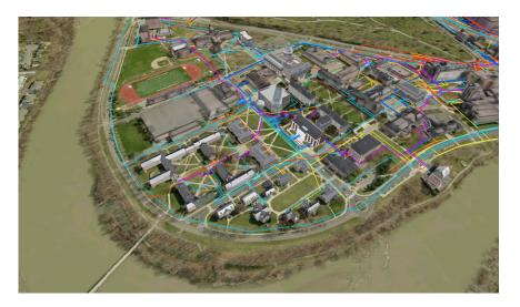
Using the ArcGIS 3D Analyst ArcGlobe software, hundreds of existing utility plans and as-built drawings were georeferenced and converted into file geodatabase feature classes in a seamless layer for each system, greatly simplifying the internal "call-before-you-dig" process. (Aerial imagery from Pictometry International)
