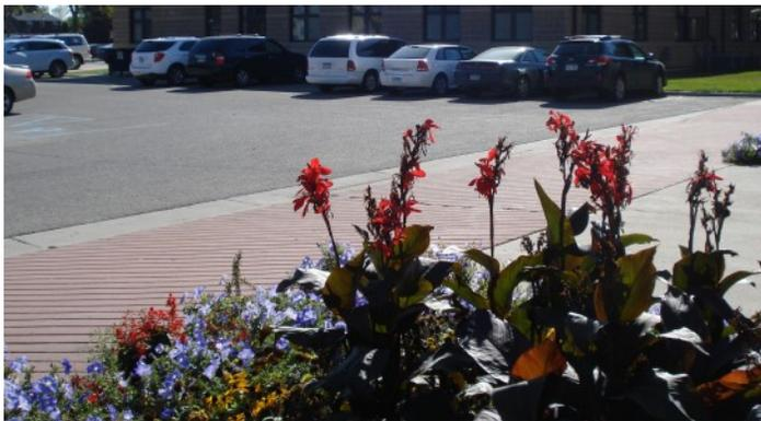
*Pavers or stamped concrete can help mark a transition between vehicular and pedestrian circulation.*
