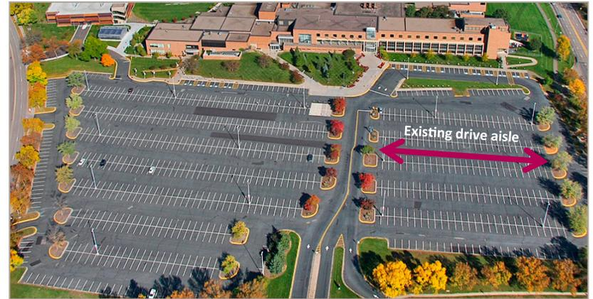
*Before: Drive aisles in this parking lot are parallel to the main building and sidewalks, creating unsafe conditions where pedestrians must walk between parked cars to get to the building entrances.*
